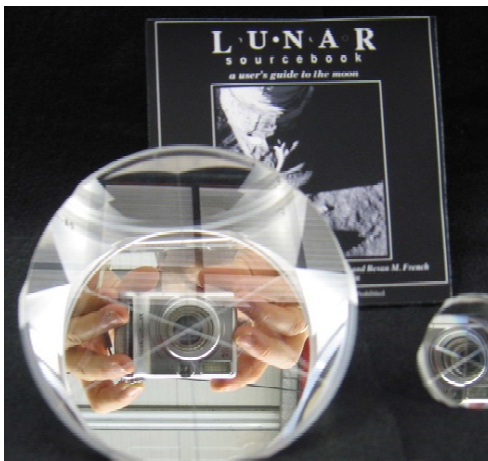
Fig. 1 Shows the Flight Certified 100 mm CCR that has been fabricated to the specifications with Apollo CCR. In fact, the offset angles for the back faces exceeded the specifications by almost a factor of two.
